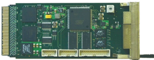
Simple MicroTCA Support Module acts as a shelf manager and provides basic system functions
