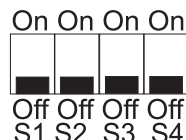
Figure 6-4 : DIP switch settings for battery backup disabled
