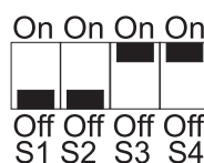
Figure 6-2 : DIP switch settings for Battery Backup by on board Lithium Cell (factory configuration)
