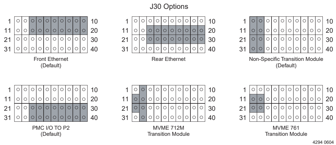
Figure 1-4 Front/Rear Ethernet Option Settings
