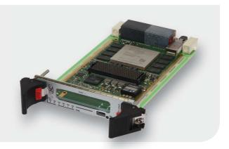
Based on the latest Xilinx 20nm FPGA family, the **IC-FEP-VPX3f** enhances the front-end processing (FEP) product line of Interface Concept, as the first VITA 66.5 compliant FPGA board on the market today.
