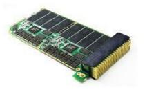
Renice 3U VPX Solid State Drive demonstrates a highlyreliable storage solution for real-time signal acquisition, processing, storage and playback. Implementations include: satellite navigation and communication, radar stations, aviation, naval, military, vehicle and off-site experiment.
