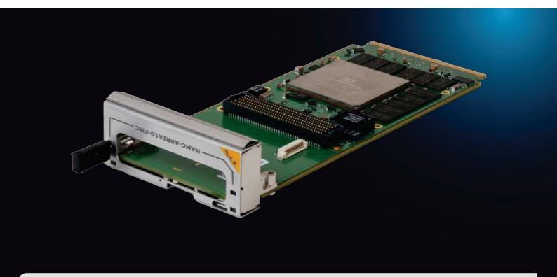
The **NAMC-ARRIA10-FMC** is an AdvancedMC (AMC) featuring the Intel® Arria® 10 GX or SX FPGA and a high pin-count FMC slot (VITA 57.1). Intel® Arria® 10 FPGAs deliver massive performance and power consumption improvements compared to prior-generation FPGAs, both midrange and high-end devices.
