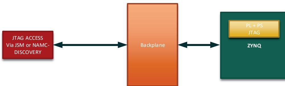
The **NAMC-ZYNQ-FMC** PS and PL JTAG Ports can be accessed using the MicroTCA Backplane JTAG signalling. In order to terminate the JTAG signals on the Host Side a JSM (JTAG switch module) is needed. For debugging and standalone debugging also a NAMC-DISCOVERY can be used to access the JTAG port.
