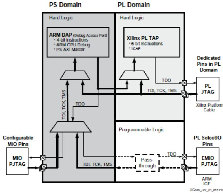
The **NAMC-ZYNQ-FMC** provides debug accesses via standard JTAG (IEEE 1149.1) debug interface in the following figure.
