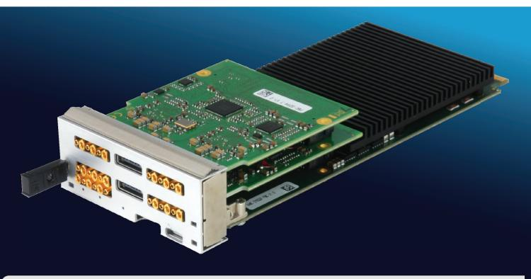
The NAT-AMC-ZYNQUP-SDR (ZYNQ Ultrascale Plus) is a flexible software defined radio (SDR) platform for wireless applications, such as mobile cellular systems with massive MIMO or radio beamforming, which require a large number of phase-coherent antennas. It can support four or eight channels, defined by the number of stacked mezzanine cards.
