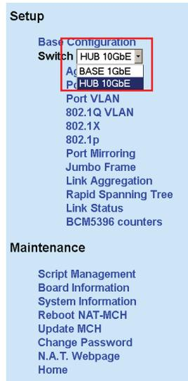
The current menu item shows the operable switch. To change the operable switch a switch device from the drop down menu has to be selected. The browser content is refreshed automatically.
