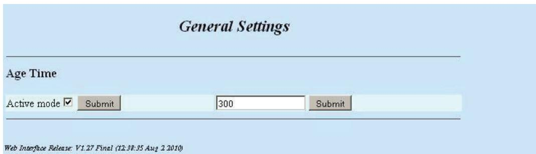
Use the <Active mode> checkbox to enable/disable the aging process and the text field to set the aging intervals of table scanning.
