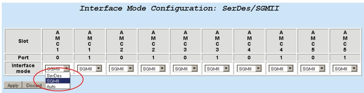
Figure 6-37: Interface mode SerDes/SGMII on AMC Backplane Ports
