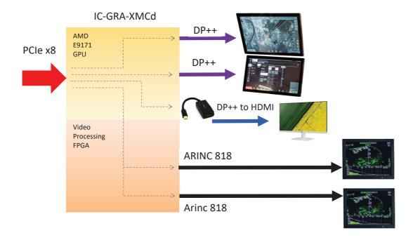
In this case, the solution takes advantage of the 2 Display Port interfaces of the 9171 GPU for very high resolution displays.
