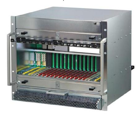
The MTCA-12S-RF2 MicroTCA® chassis is a 9U 19" rack offering up to 12 AdvancedMC™ slots, all are MTCA.4 compliant slots with µRTMs. The MTCA-12S-RF2 system is the perfect base for complex and highly integrated computer platforms in high energy physics applications. It supports high-end computing applications as well as I/O intensive configurations. Based on the MicroTCA® and AdvancedMC™ PICMG® standards it is the optimal solution for long life cycle applications.
