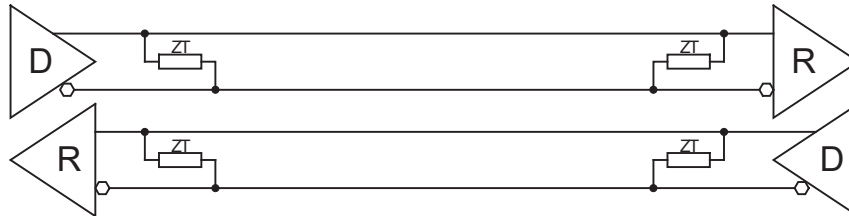
Figure 5-11: RS485 Full Duplex Point to Point Configuration
