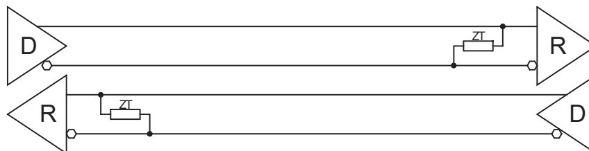
Figure 5-5 : RS422 Full Duplex Point to Point Configuration
