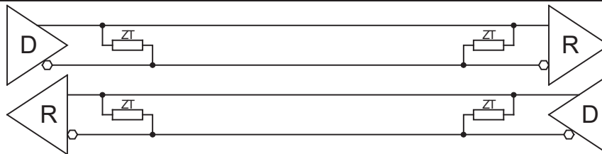
Figure 5-6 : RS485 Full Duplex Point to Point Configuration
