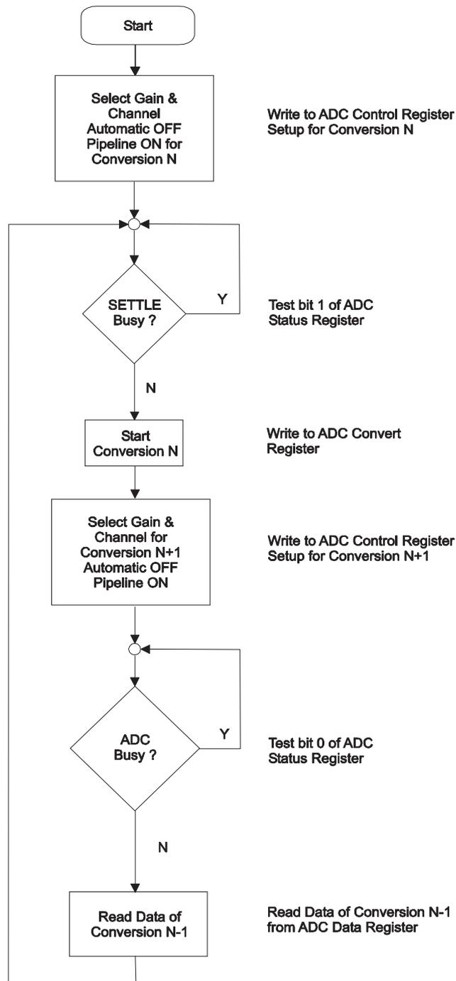
Figure 5-2 : Normal Mode with Data Pipeline Flow
