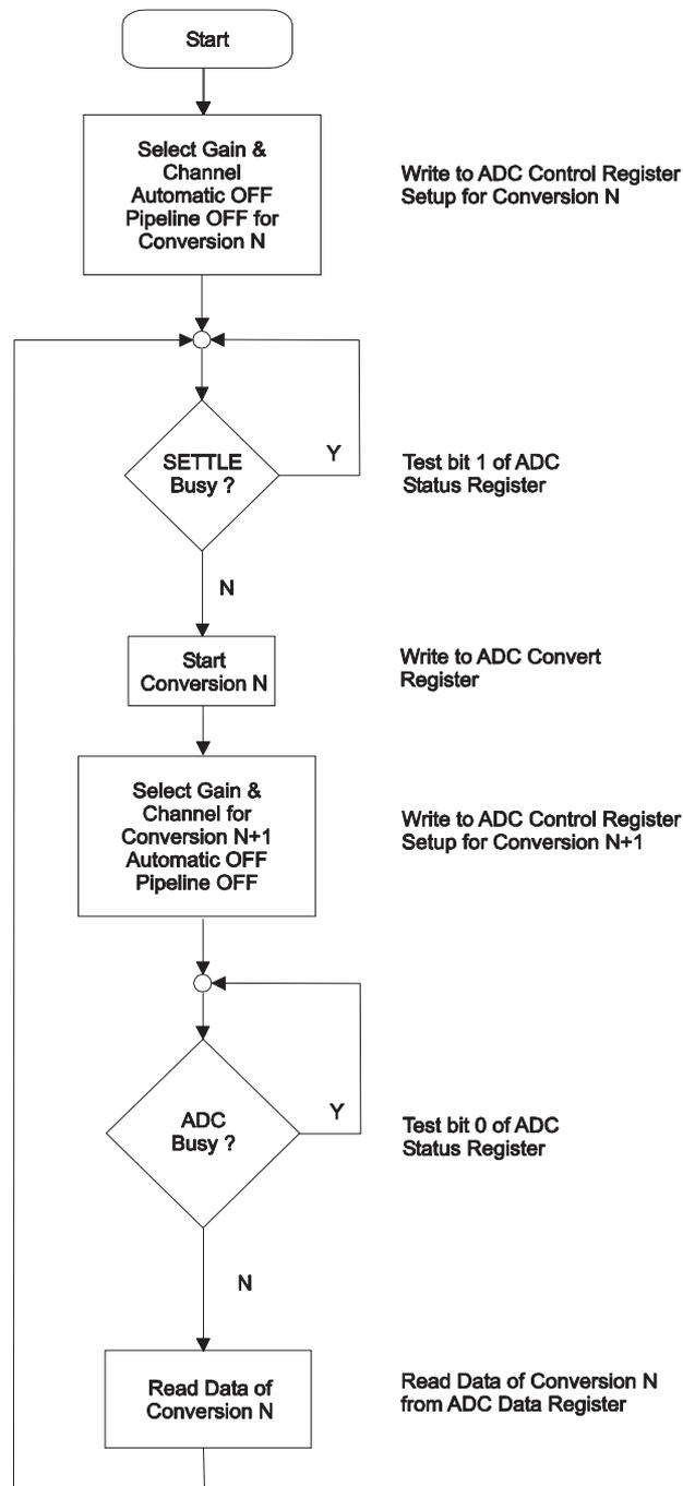
Figure 5-1 : Normal Mode without Data Pipeline Flow
