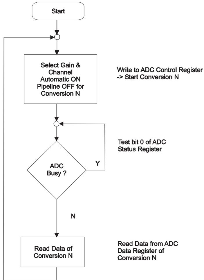
Figure 5-3 : Automatic Mode without Data Pipeline Flow
