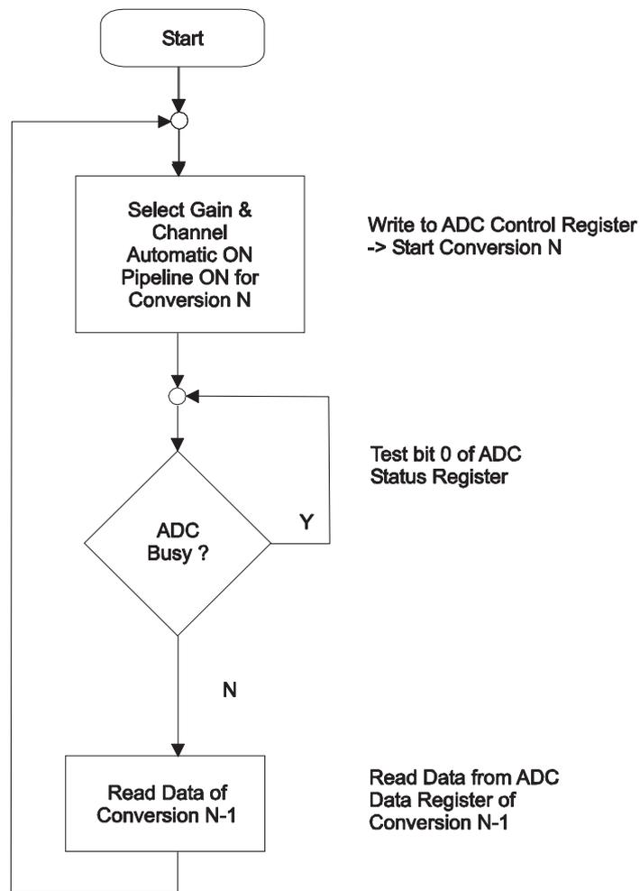
Figure 5-4 : Automatic Mode with Data Pipeline Flow
