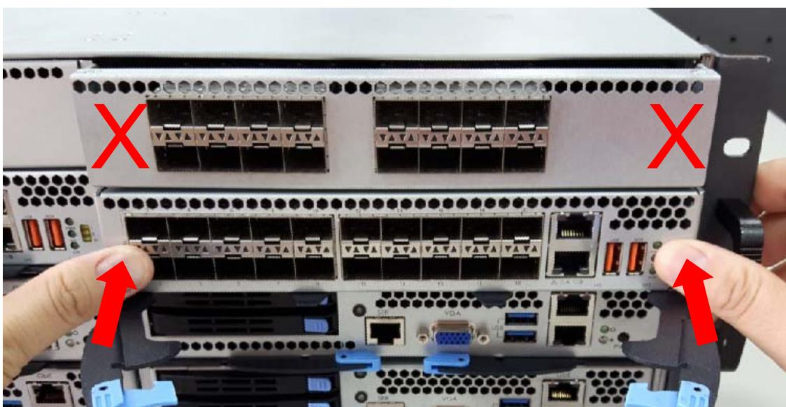
3. When the Switch sled is fully inserted into the chassis, the locking handles will be pulled into the closed position and the front panel will be flush with the chassis.
