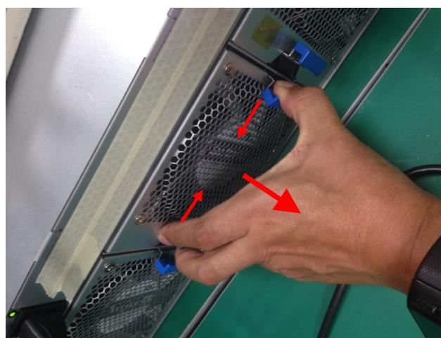
2. Align the new fan module so that the arrows and “TOP” markings are as shown below. Insert the fan into the fan slot and press firmly until both fan ejector latches are secured.
