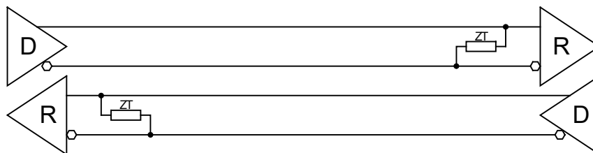
Figure 5-5 : RS422 Full Duplex Point to Point Configuration
