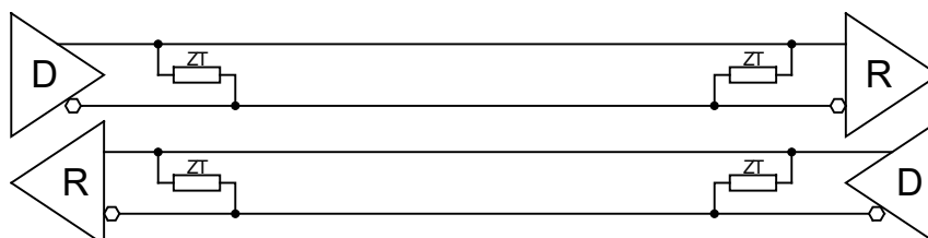
Figure 5-6: RS485 Full Duplex Point to Point Configuration
