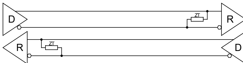
Figure 5-5: RS422 Full Duplex Point to Point Configuration
