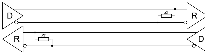
Figure 5-5 : RS422 Full Duplex Point to Point Configuration
