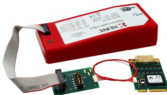
Figure 7-2: TMPE623 connected to a Programmer via TA308
