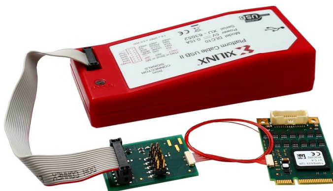
Figure 7-5 : TMPE633 connected to a Programmer via TA308
