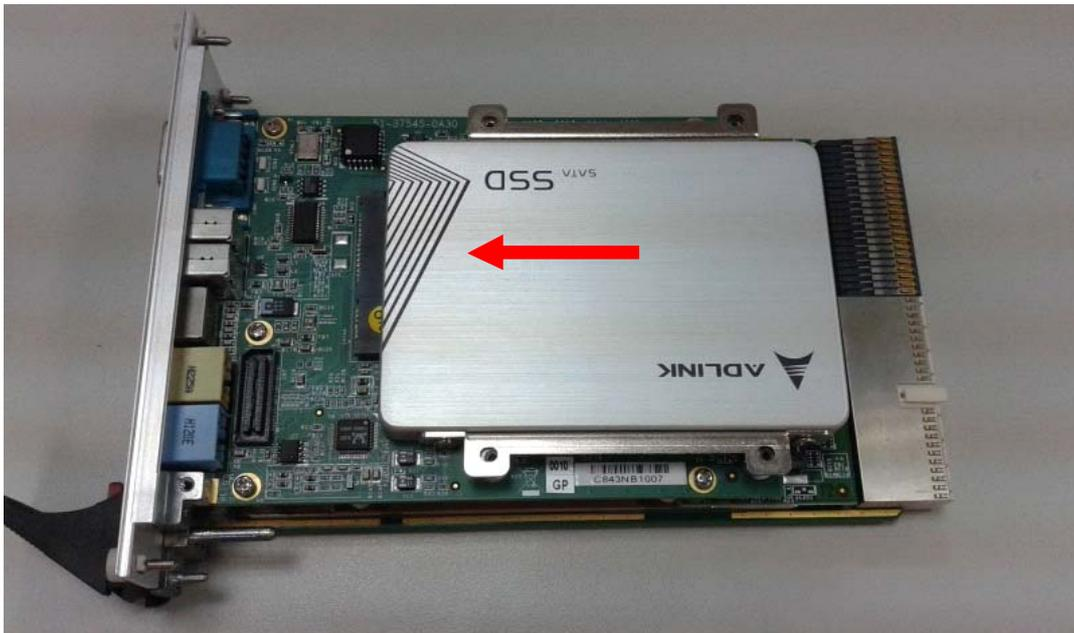
5. Secure the hard drive assembly to the cPCI-3510 with four M2.5 screws provided.
