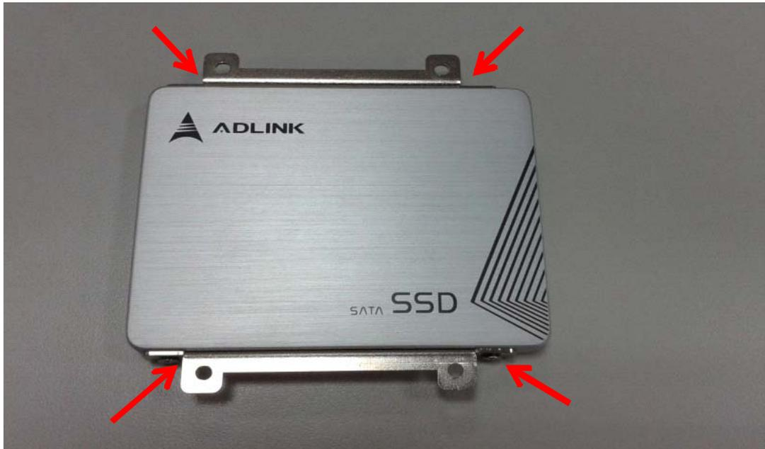
4. Align the drive assembly with the cPCI-3510 and insert it into the onboard SATA connector until it is properly seated.
