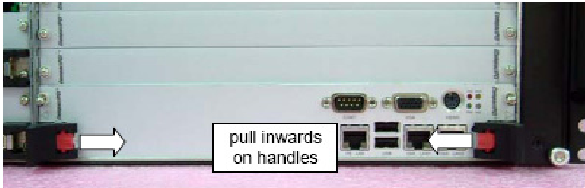
Figure 2-2: Latching the cPCI module handles securely.
