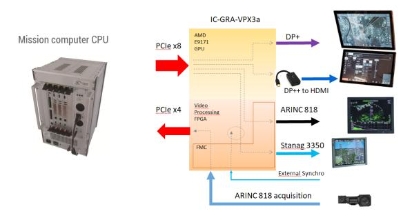
In this case, the mission computer CPU takes advantage of the 2 Display Port interfaces of the 9171 GPU for very high resolution displays (one in DP+ mode, and the second one in HDMI mode via a DP+ to HDMI converter).
