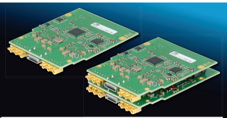
The NAT-FMC-SDR4 is a radio frequency (RF) front-end FMC module that provides eight front panel ports for connection to antennas in wireless networks (4x transmit, 4x receive). ADRV9009 RF transceivers provide the transmit/receive functionality, with 200 MHz instantaneous bandwidth per channel. It provides a platform for wireless applications, such as mobile cellular systems with massive MIMO or radio beamforming, which require a large number of phase-coherent antennas.
