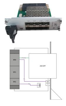
**RTM19** is a 3U VPX real transition module to be coupled with **ComEth4590a** control plane:
