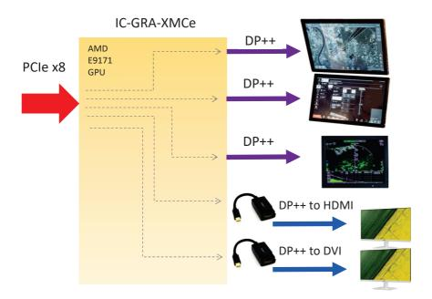
In this case, the solution takes advantage of 3 Display Port interfaces of the 9171 GPU for very high resolution displays.
