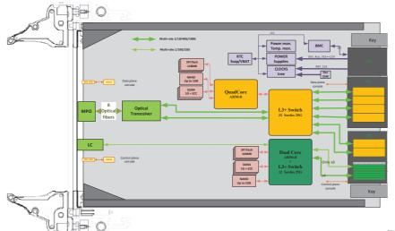
The **ComEth4690e** is compliant with VITA 65.0 Slot Profile SLT3-SWH-6F1U7U-14.4.14.
